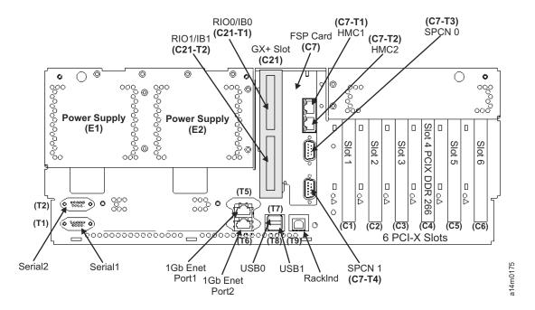
Figure 12. IBM TS1120 (3592 C06) Controller back panel
