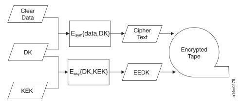
Figure 5. Encryption with both symmetric and asymmetric encryption keys
