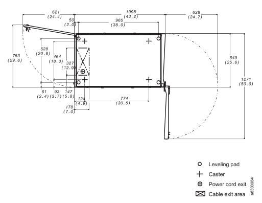
Figure 13. Top View of 3952 Model F05 Frame Layout
