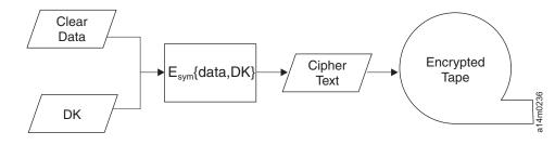
Figure 6. Encryption with only symmetric encryption keys
