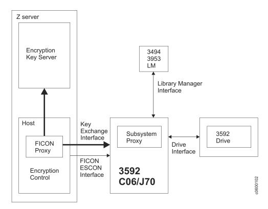
Figure 3. In-band encryption key flow
