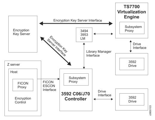
Figure 4. Out-of-band encryption key flow
