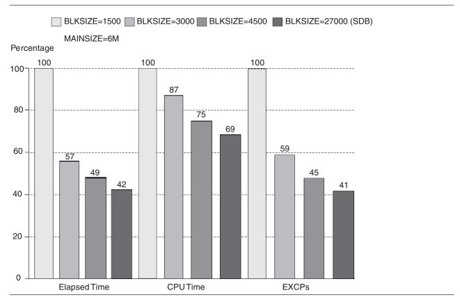
Figure 8. Benefits of Large Input/Output Data Set Block Sizes
