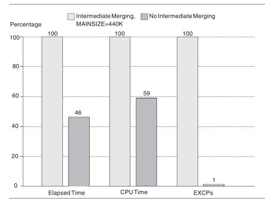
Figure 6. Benefits of Eliminating Intermediate Merging
