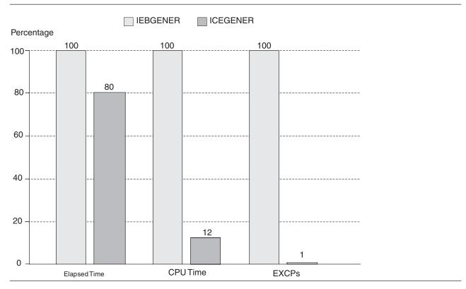
Figure 1. ICEGENER versus IEBGENER Copy Comparison
