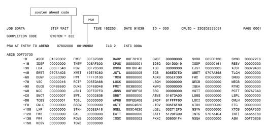
Figure 3. Finding the System Abend Code and the PSW in the SYSUDUMP
