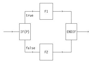
In this figure, the test of the predicate *p* is represented by the IF macro, which determines whether process F1 or F2 is to be executed. The exit path from the macro is represented by the terminator ENDIF macro. The general IF macro set is written:
