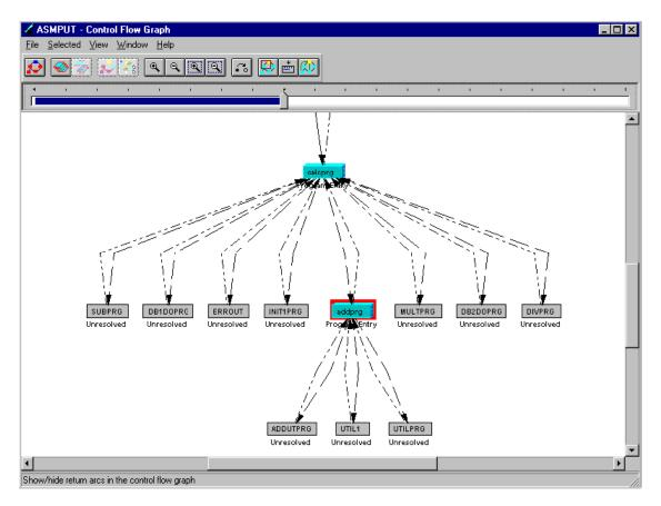
Figure 22. A control flow graph with the return arcs displayed
