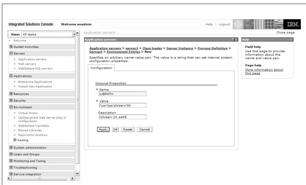
Figure 27. Adding the PKI Services shared library's location to the server's library path
