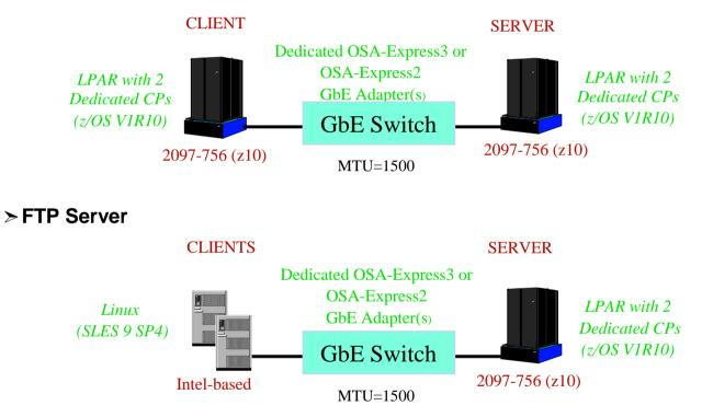
▶ All measurements were collected on a z10 (2097-756 2 CPs Client/Server LPARs) and z/OS V1R10
