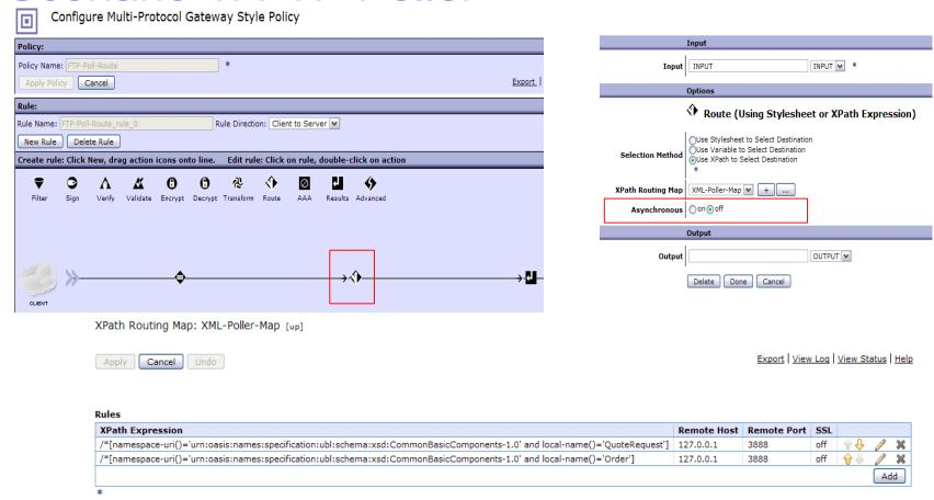
The Route Action uses an Xpath Routing Map keyed on the root node of the request to determine destination.
