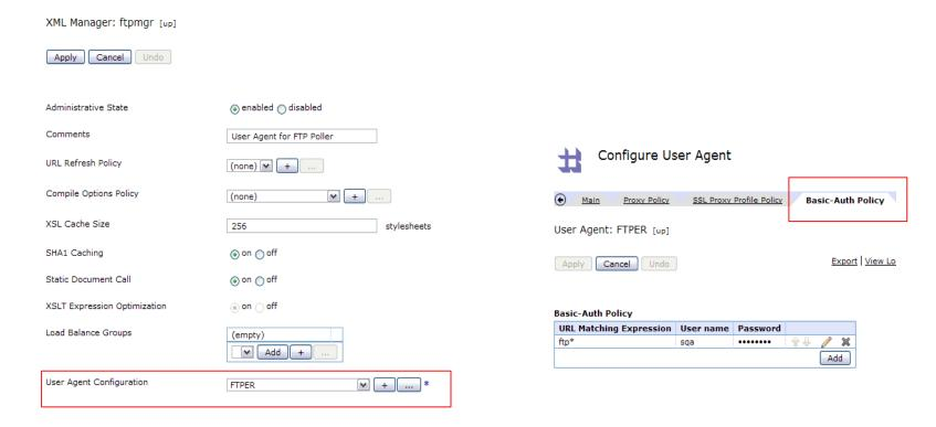
The Basic-Auth Policy of the User Agent associated with the XML Manager in use provides the credentials necessary to connect to the destination (back end) FTP Server.
