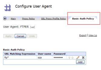
The Basic-Auth Policy of the User Agent attached to the XML Manager provides credentials for connecting to the remote FTP Server.
