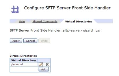
This Server FSH uses a virtual ephemeral filesystem, obscuring the file/directory structure of the destination server. This server also authenticates clients by using a public key exchange.
