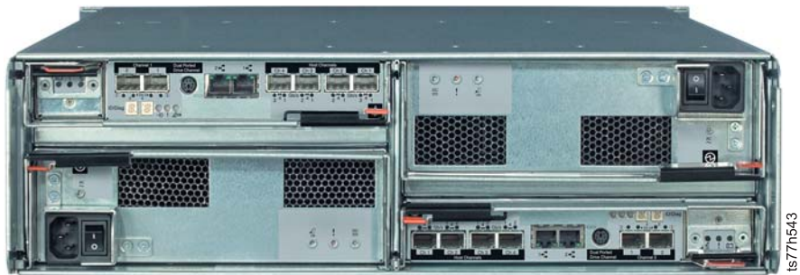
Figure 14. TS7720 Cache Drawer 3956-XS7 (rear view )
