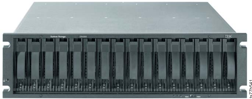
Figure 15. TS7720 Cache Drawer 3956-XS7 (front view)
