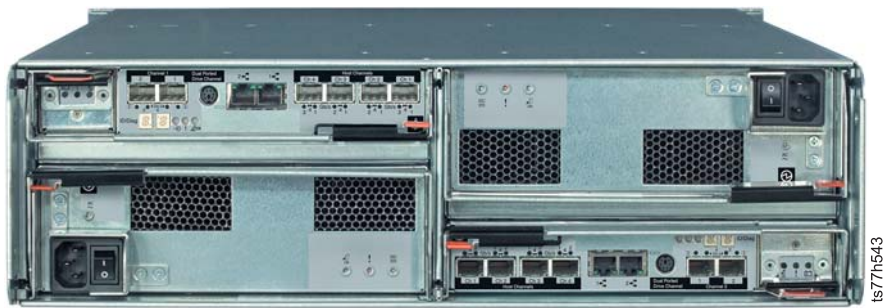
Figure 18. TS7740 Cache Controller 3956-CC7 (rear view)
