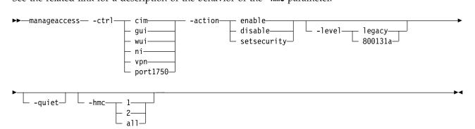
The following diagram shows the **manageaccess** command with the **-ctrl** parameter value set to **vpn**.
