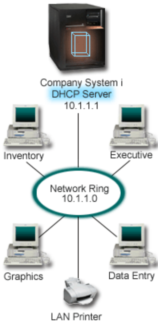
Figure 2. Simple LAN setup for IBM i model
