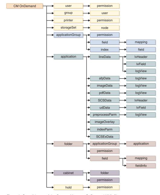
Figure 6. Overall layout of the Content Manager OnDemand XML file
