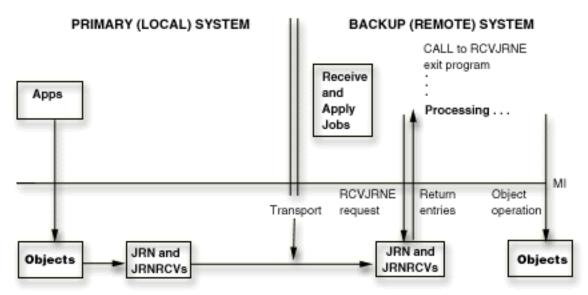
This figure above illustrates that processing with the remote journal function occurs synchronously to the operation that is causing the journal entry deposit. This processing requires less overhead than the RCVJRNE command.
