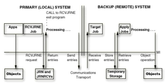
This figure above illustrates that processing with the RCVJRNE command occurs asynchronously to the operation that is causing the journal entry deposit. This processing requires more overhead than the remote journal function.
