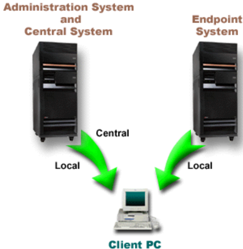
Figure 3. The administration system and the central system can be the same system. It does not change the function of Application Administration or Management Central. When a Client PC connects to a system, the Local Settings come from the system that you connect to. When you connect to an administration system, the Central Settings are sent to your Client PC from the administration system.
