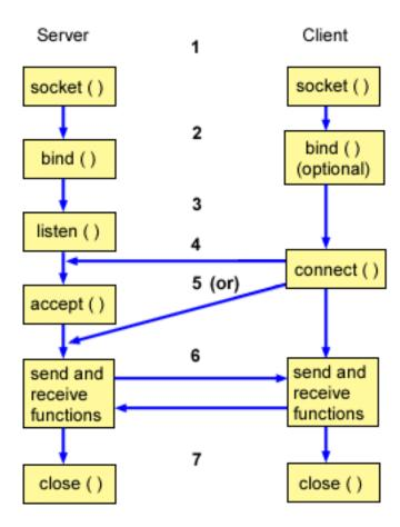
This is a typical flow of events for a connection-oriented socket:
