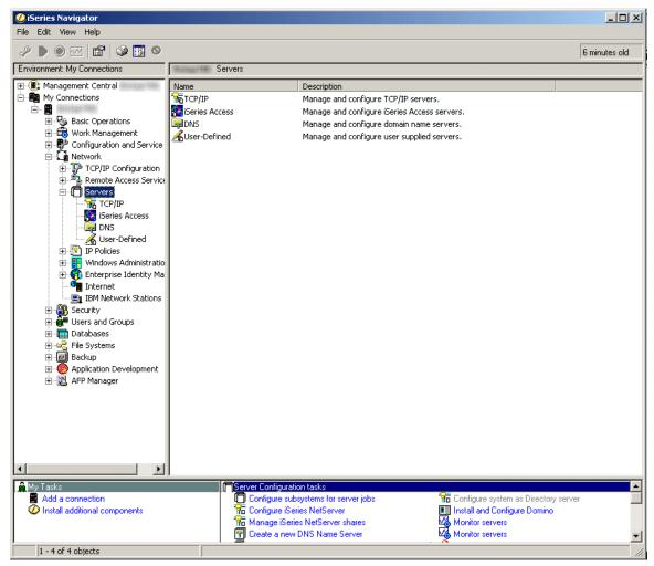
6. Select the type of servers that you want to configure subsystems for. DDM and iSeries NetServer are TCP/IP servers. Central, Database, Data Queue, Files, Net Print, Remote Command, and Sign On are iSeries Access servers. The remaining steps use a subsystem from iSeries Access. The subsystem configuration steps are identical for each server.
