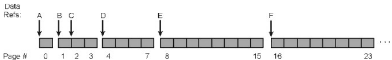
Figure 20. Sequential Read-Ahead Example
