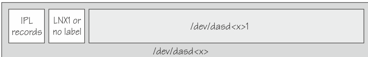
Figure 54. Linux disk layout
