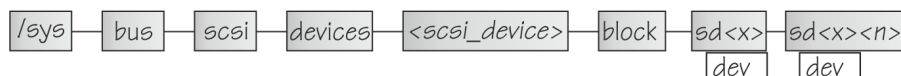
Figure 64. Major and minor numbers for block devices that correspond to SCSI disks in sysfs
