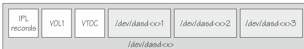
Figure 53. Compatible disk layout
