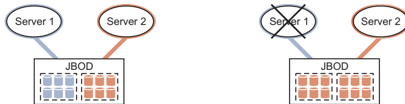
Figure 5. Minimal configuration of two GPFS Native RAID servers and one storage JBOD. GPFS Native RAID server 1 is the primary controller for the first recovery group and backup for the second recovery group. GPFS Native RAID server 2 is the primary controller for the second recovery group and backup for the first recovery group. As shown, when server 1 fails, control of the first recovery group is taken over by its backup server 2. During the failure of server 1, the load on backup server 2 increases by 100% from one to two recovery groups.
